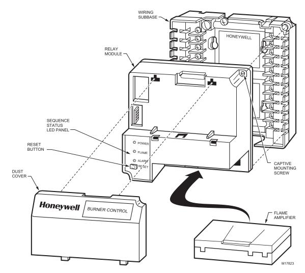
Fig. 3. EC/RM7823A Relay Module, exploded view.
