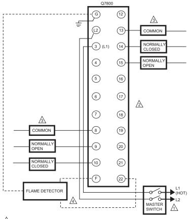
3 OUTPUTS SHOWN ARE WHEN THE DEVICE DOES NOT SEE FLAME.
