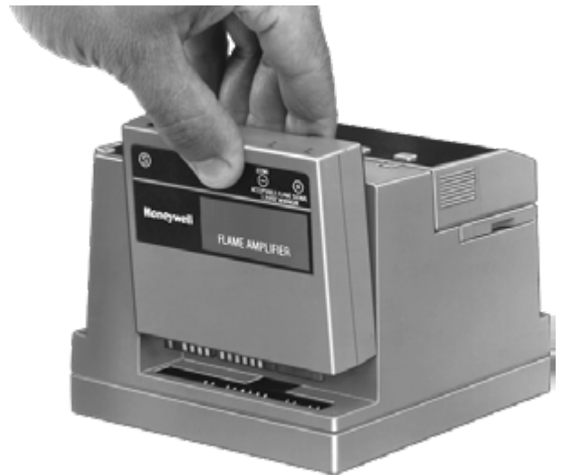
Fig. 2. Installing flame signal amplifier.
